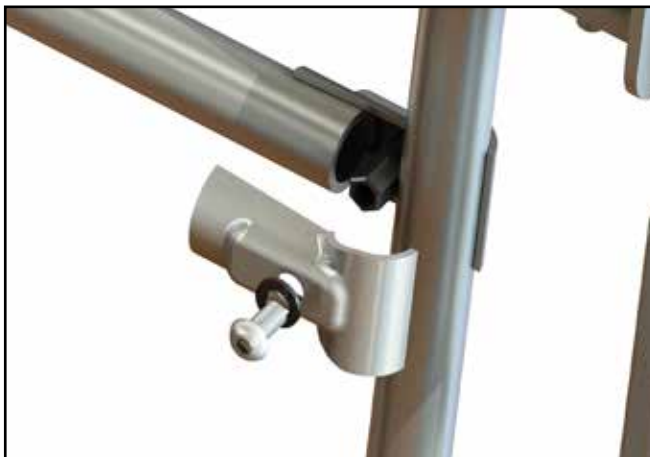
P. Add clamp onto other end of mid rail, clamping onto the gate upright. Use 6mm hex head socket to tighten supplied M10 bolts into coupling nut.
