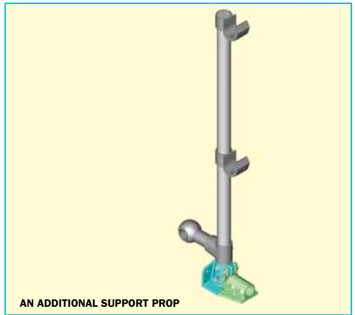
A HINGED VERSION OF THE STANDARD KEEGUARD BASE FITTING
