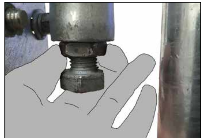
K. To tension the hinge loosen the locking nut as shown.
