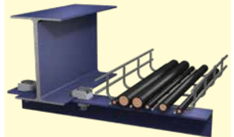
Cantilevered angle support to I-Section
