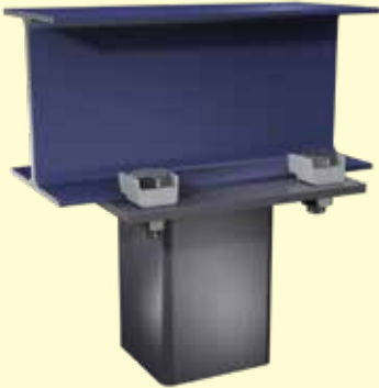
Column end plate to I-Section
