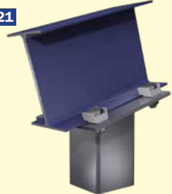
Column end plate to sloping I-Section
