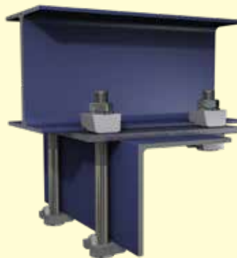
Angle section below an I-Section at 90 degrees
