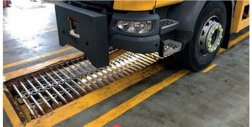
Robust yet lightweight inspection pit covers are easy and quick to deploy to protect pits.
